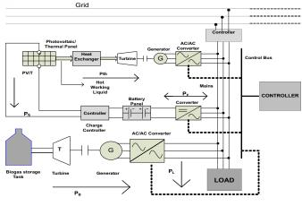
Figure 3. Complete block diagram of phtovoltaic/thermal and blogas DSP
