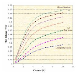
Figure 7: Flux linkage versus current for 4 phase, 8/6 poles base srm.
