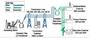
Figure-1: A typical Power System [2].
