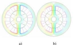
Figure 6: Flux distribution in 4 phase, 8/6 pole SRM a) Base design; b) Optimized design
