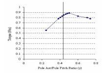
Fig. 3. Torque versus pole arc/pole pitch ratio (ã)
