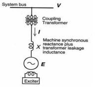
Figure-5: Reactive Power generation by a rotating synchronous compensator [2].
