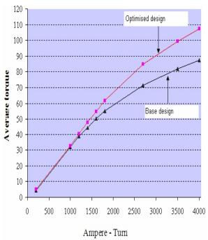
Figure 5: Average torque versus ampere-turns for 4 phase, 8/6 poles base and optimised srm.
