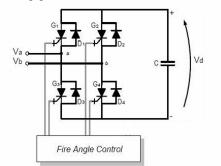
Figure 7. Three-Pulse Voltage Source Converter [2].
