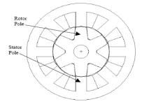
Fig. 1b: Cross section for 4 phase, 8/6 poles Reference (or base) SR motor
