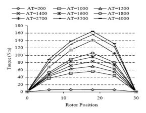
Fig.1c: Torque versus rotor position at different MMFs
