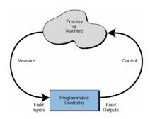
Fig. 1 PLC Conceptual Application Diagram
