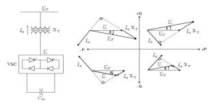
Figure 9. Phasor Diagram of STATCOM [2].
