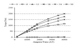
Fig. 2c: Torque versus MMFs at different rotor angles
