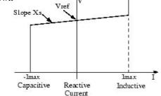
Figure 10. V-I Characteristics of STATCOM [1].
