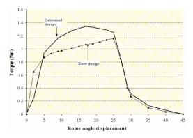
Figure 11: Torque versus è for Base SRM and Optimised SRM.
