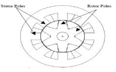
Fig. 2a: Optimised SR motor configuration
