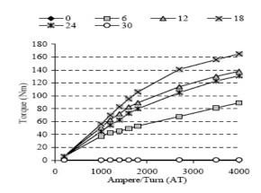
Fig. 1d: Torque versus MMFs at different rotor positions.
